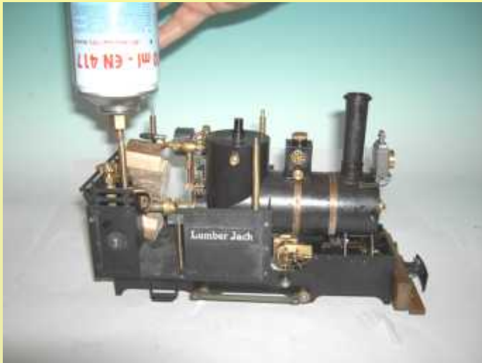
Filling gas with the one-hand gas fill adapter
